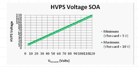
The "HVPS Voltage SOA" graph shows the full range of adjustability for the HVPS that is set based on the forward voltage of the laser being driven. Operation of the instrument outside of this range can result in permanent damage to the instrument, laser or both.
