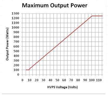
The graph above shows the maximum output power of the instrument for all HVPS voltage settings. Operation of the instrument above the graphed limit can result in permanent damage to the instrument, laser or both.
